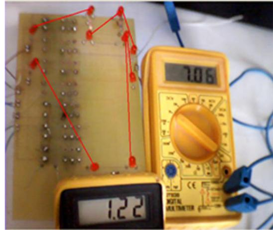
Fig. 1 A virtually wired real circuit in the AR remote lab leads to AR based visualization.
